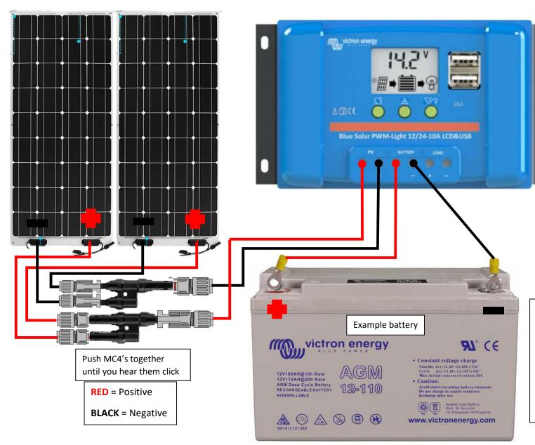
Connect the battery cables first, then the solar.
